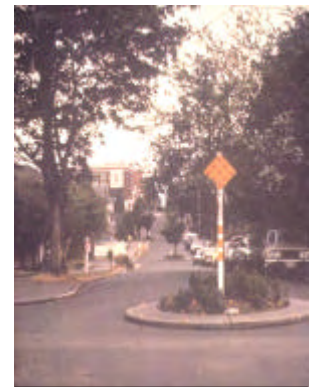
Traffic circles and other devices such as textured surfaces, raised intersections and neckdowns are techniques that reduce vehicle speeds and help manage traffic in downtowns and on local neighborhood streets.
